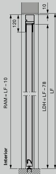
Side door with aluminium block frame, profile type 2 Fitting in the opening
